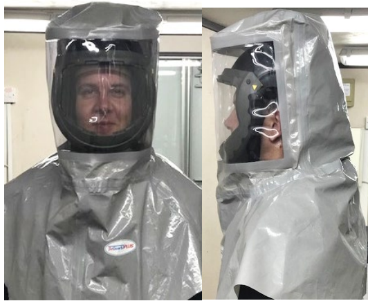
Fig.5 A chemical over-hood will not only provide splash protection during use but prevent damage and minimise cleaning to the respiratory equipment.
